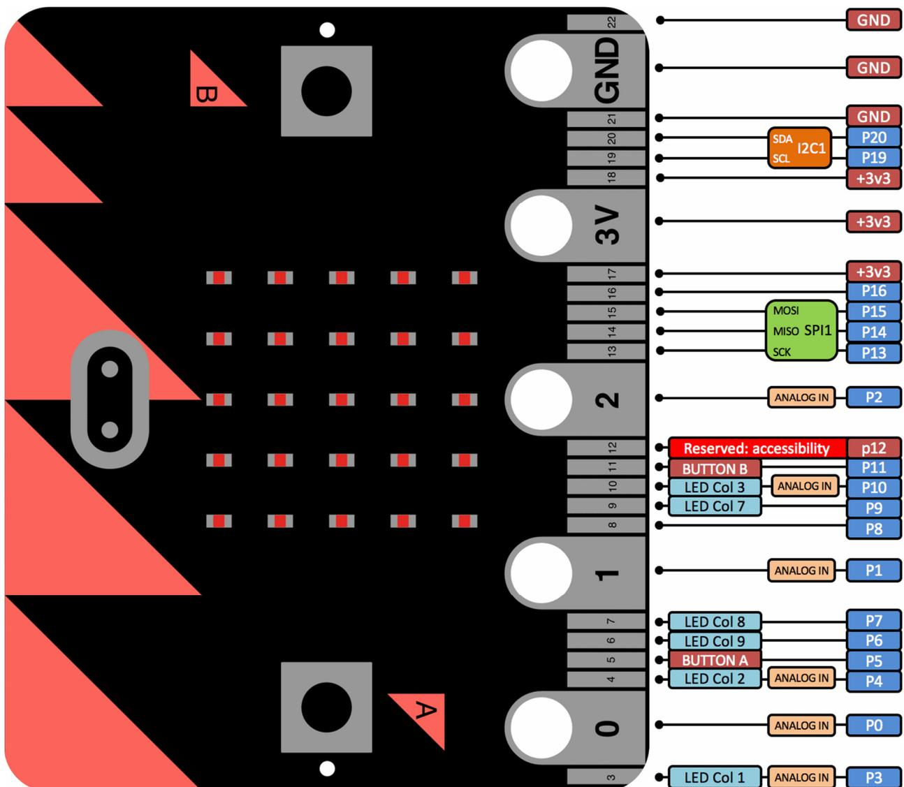
The micro:bit has 25 external connections on the edge connector of the board, which we refer to as 'pins'. The edge connector is the grey area on the right side of the figure above.
